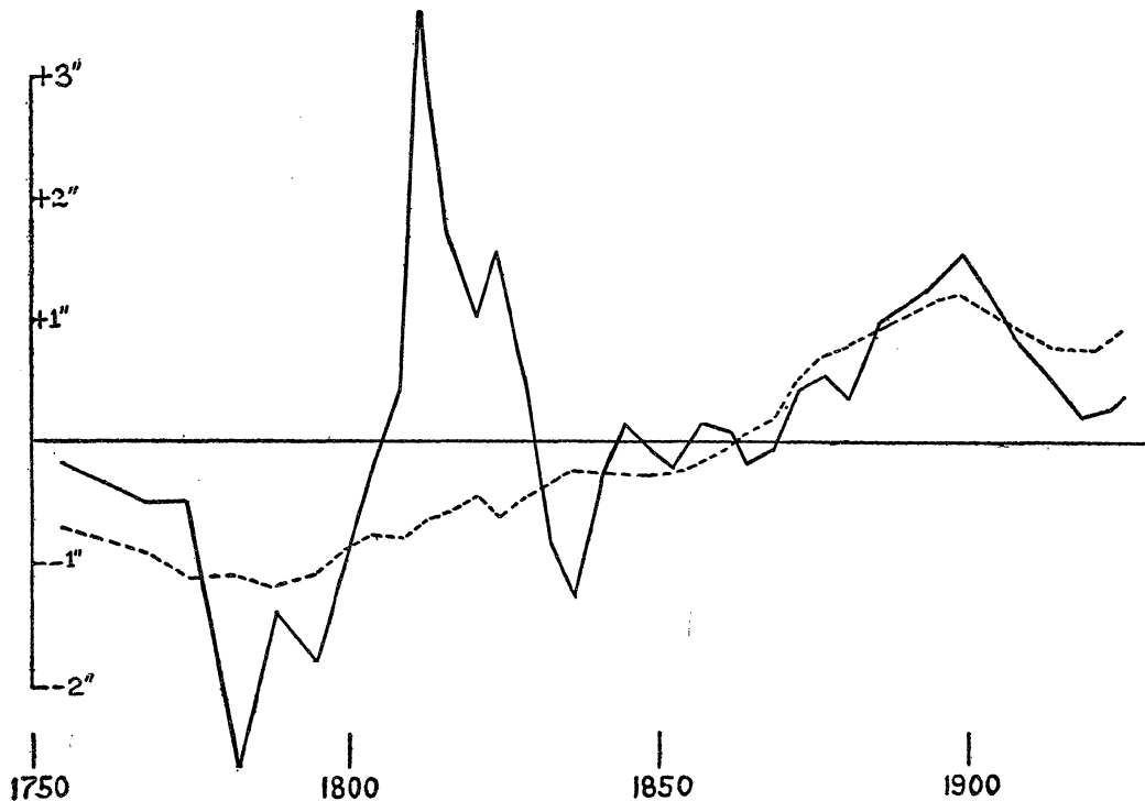
FIG. 4. Full line curve: the Greenwich tabular minus observed errors of the Sun including the secular acceleration. Dash line: 1/13.3 of the lunar fluctuations.
